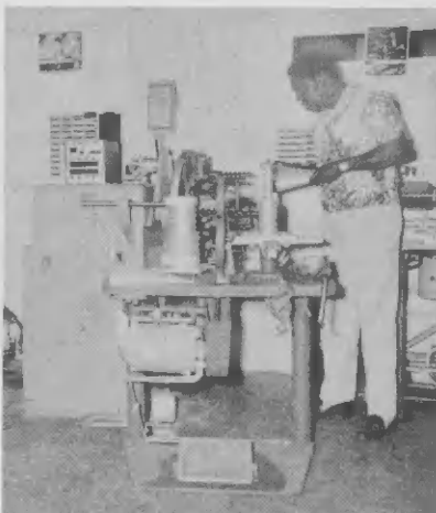
Ricardo Croes makes adjustment on new coil winding machine. The old winding machine is at left. At right, Supervisor Arnold Beyde shows various types of winding heads of the winding machine and also the new coil taping machine, in front.
